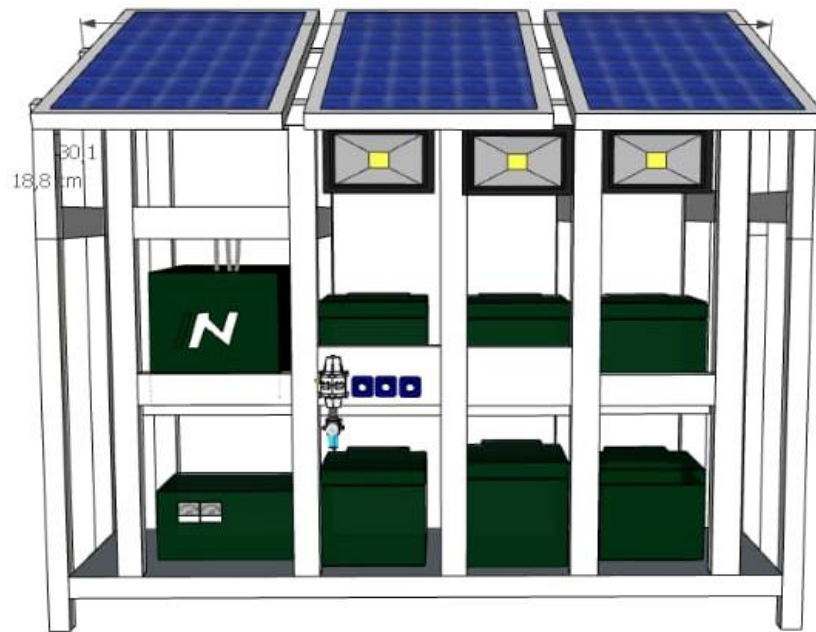
Gambar 3. 3 3d Desain SketchUp Panel Surya
