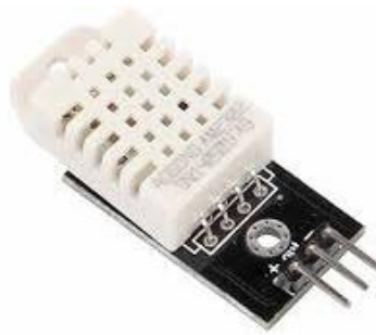
Gambar 2.3 Sensor DHT22 (Srivastava, et al., 2018)
